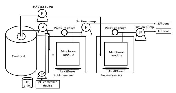
Fig. 3 - Membrane bioreactors used in this study.
