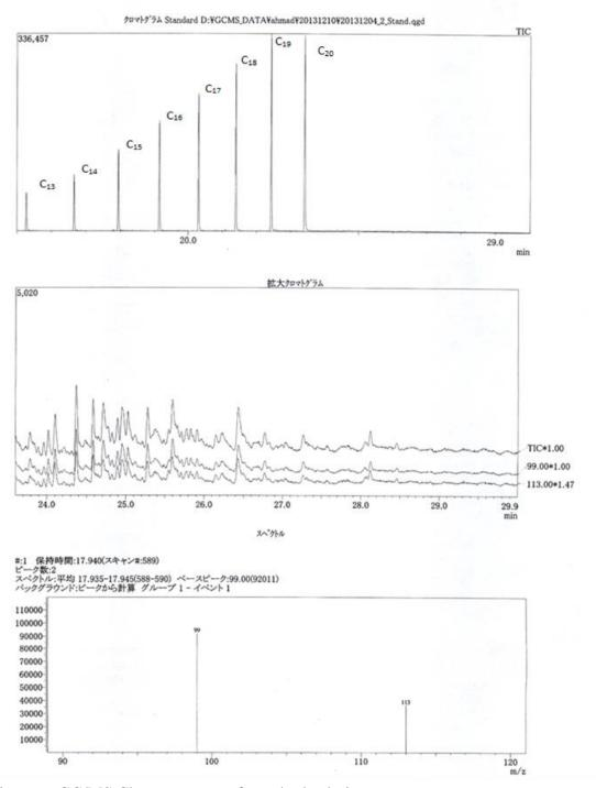
Figure 6: GC/MS Chromatogram of standard solution.
