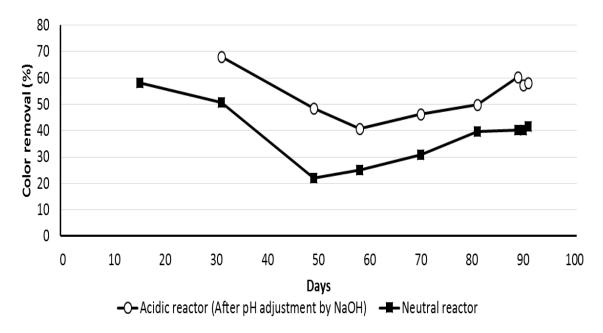
Fig. 12 - Change in the percent removal of color measured at 390 nm.
