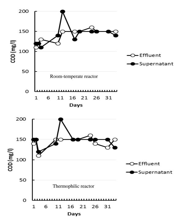
Fig. 18 - COD of effluent and the supernatant of the mixed liquor of activated sludge.
