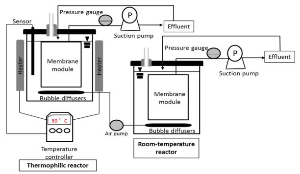
Fig. 4 – Schematic diagram of the membrane bioreactors.
