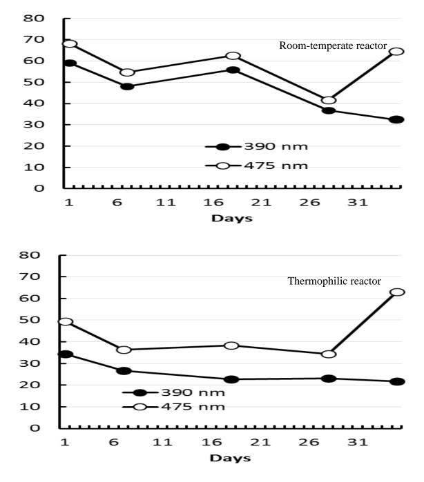
Fig. 19 - Change in the percent removal of color measured at 390 nm and 475 nm.
