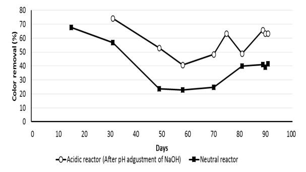
Fig. 13 - Change in the percent removal of color measured at 475 nm.
