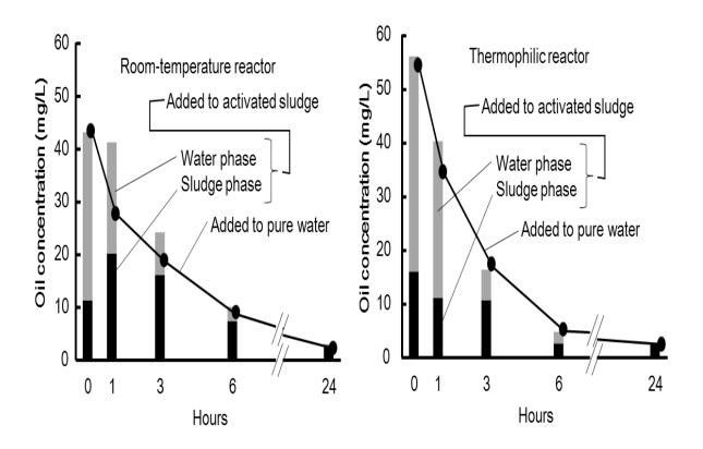
Fig. 20 – Changes in oil concentration during 24 hours after the addition of oil.
