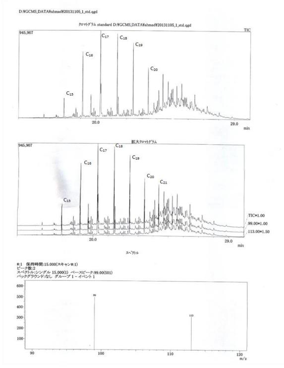
Figure 5: GC/MS Chromatogram of mineral oil used in this study.
