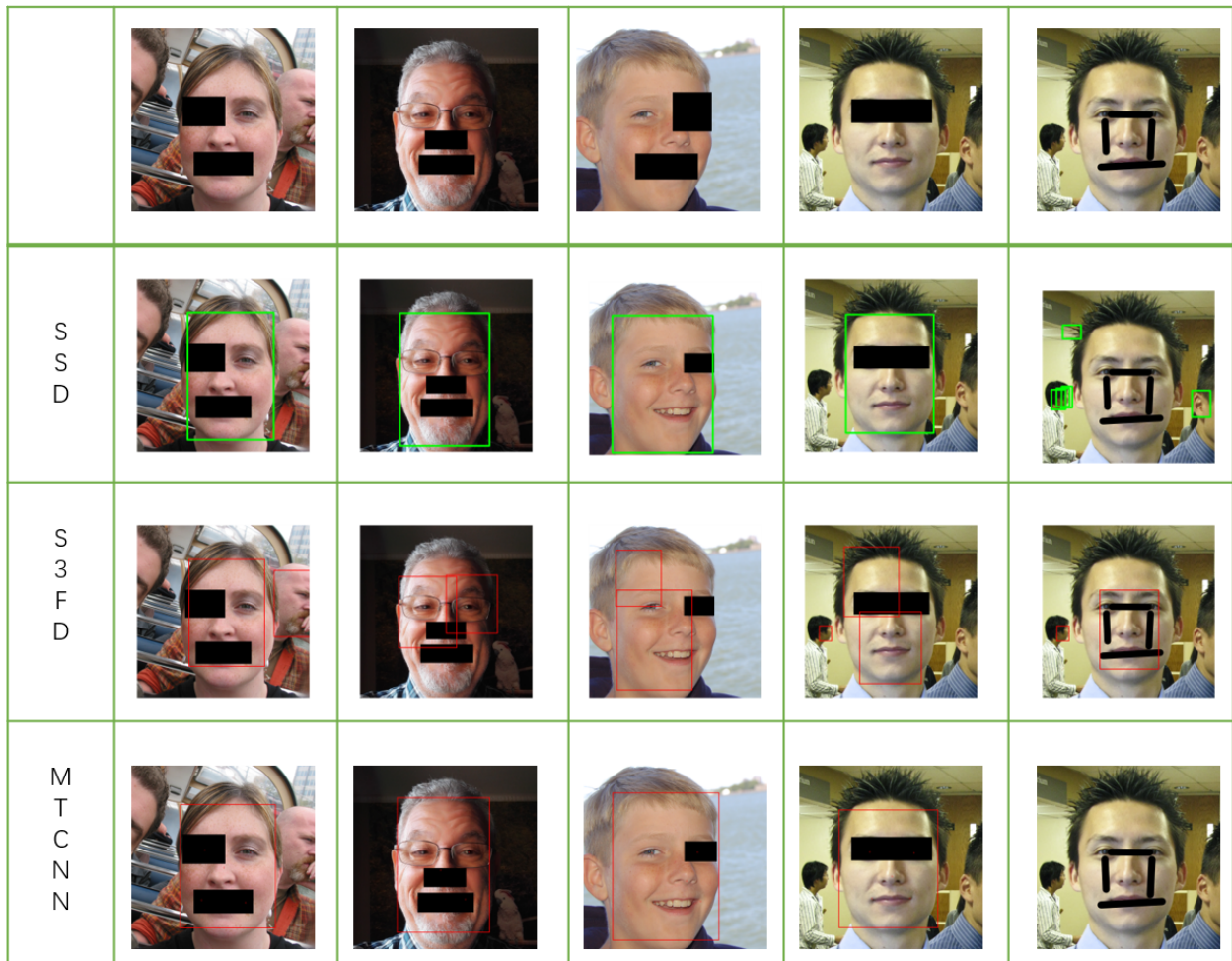
Figure 5.1: Blocking part of the facial area and performing face detection through face detectors SSD, S3FD, and MTCNN.
