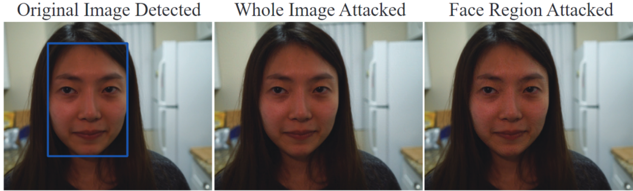
Figure 4.1: In the digital domain, attacks against whole images and faces can disable SSD-based face detectors.
