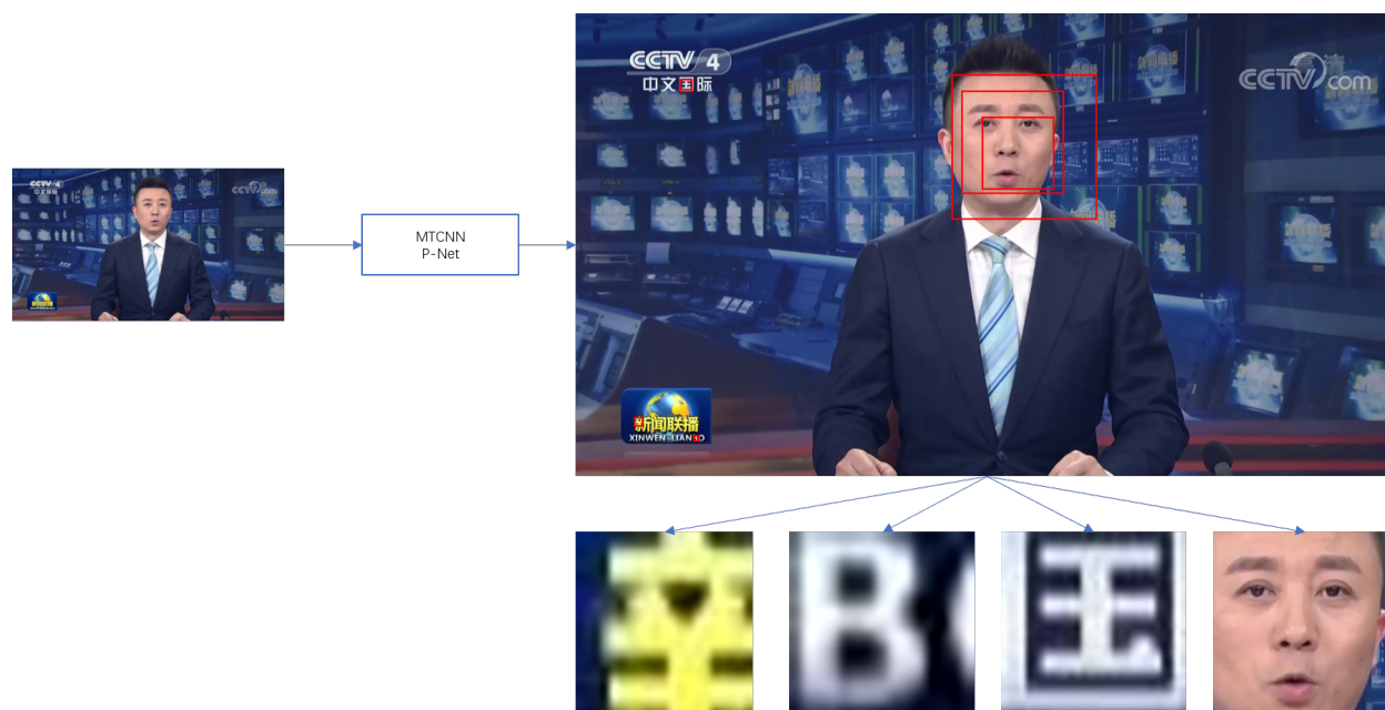
Figure 3.3: MTCNN's P-Net network for rough detection and extraction of the bounding box content.
