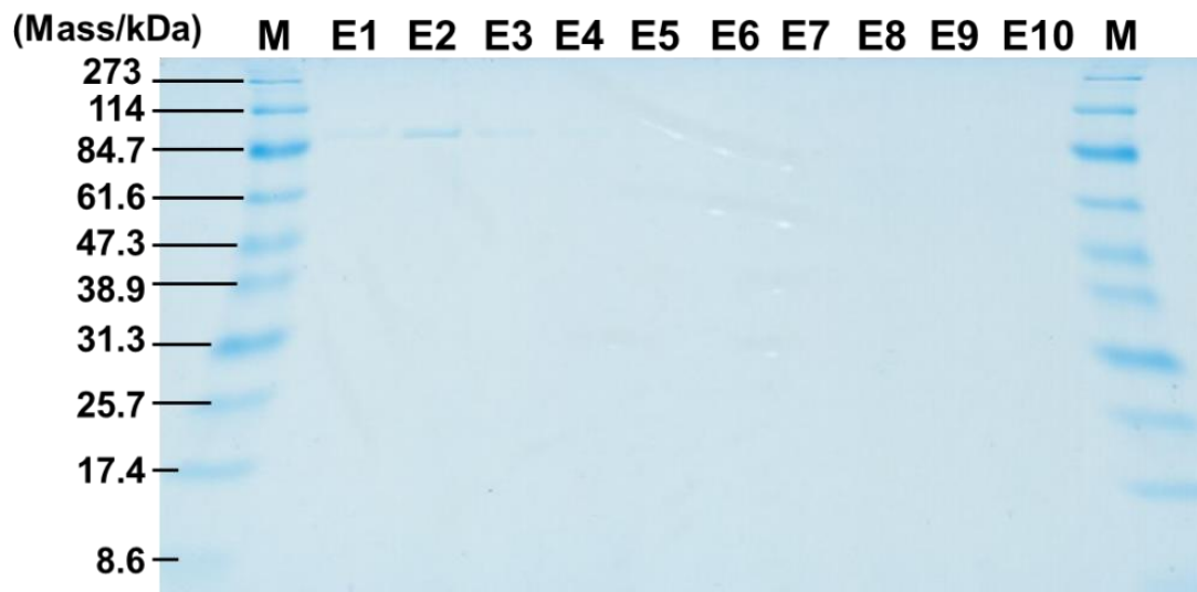
Fig. 2-10 SDS-PAGE analysis of purified UHRF1 SRA-Fluc (MW: 8.4 \times 10^4 ) The elution fractions (E1–10) were analyzed using 12% SDS-PAGE electrophoresis.
